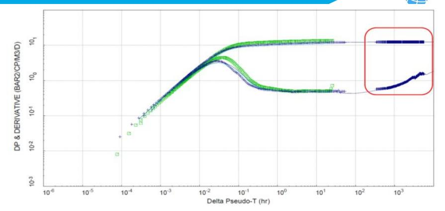
Log-log derivative plot covering the initial DST and extended pressure buildup (from SPE-180008-MS) obtained by remote sensing – not necessarily Interference testing, but demonstrates a method for achieving similar results.
