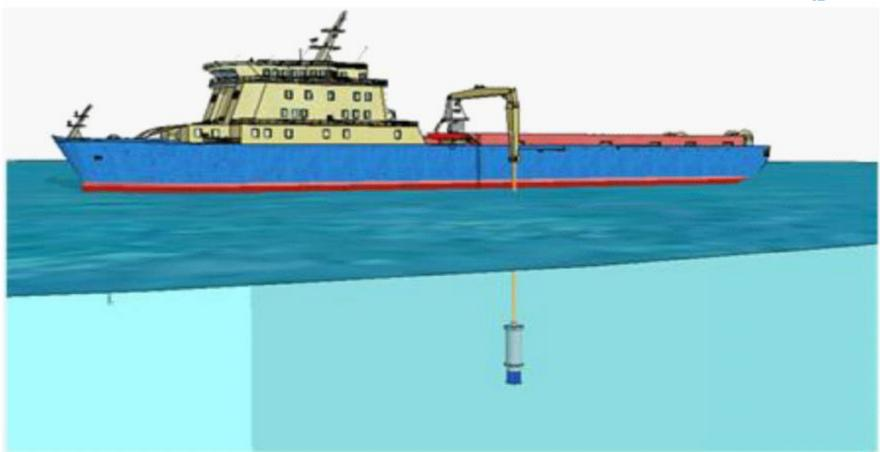
Subsea data recovery with acoustic "dunking" sonde deployed to 10-15m below sea level (from SPE-180008-MS - Norvarg field)
