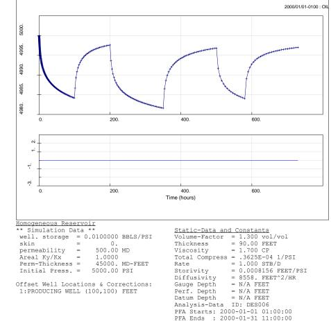
The plot on the left represents the measured response in the observation well, caused by the interference of the producing well. Values of storativity and mobility are obtained by deriving the type-curve model that matches the data and defines the reservoir properties
